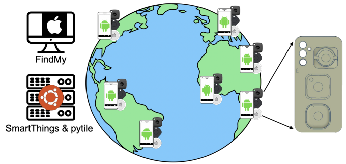
Fig. 1. On the left, two data collection servers (MacOS and Ubuntu) run the FindMy, SmartThings, and pytile crawlers. On the right, a sample 3D mockup of our vantage point, a Galaxy A34 equipped with three tags.
